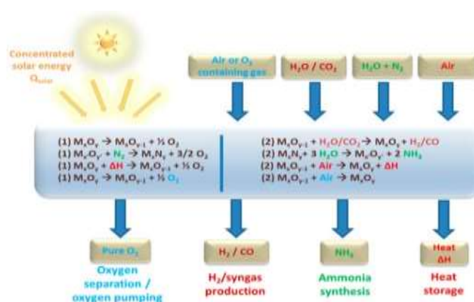
Figure 1. Metal oxide redox cycles applied to solar chemical processing involving thermochemical oxygen separation/oxygen pumping, fuel production (H 2 , CO), ammonia synthesis, and thermochemical energy storage. https://www.mdpi.com/1996-1944/16/9/3582
