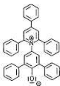
Solvatochromic Betaine Dye for the Determination of Empirical Parameter of Solvent Polarity [ E_T(30) and E_T^N ]
